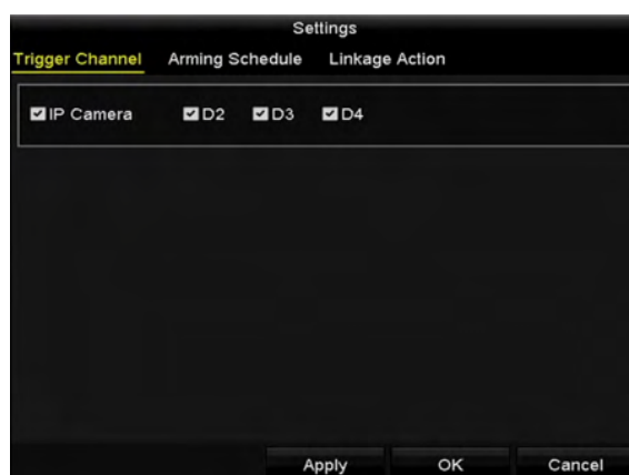
Figure 5-17 Set Trigger Camera of VCA Alarm
